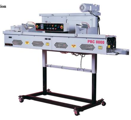
A valuable addition to any semi- or fully automated packaging line, the PBC 8000 features a maintenance free, variable speed, direct drive system. Three independently controlled heat zones close pre-glued bag flaps up to 6,4 cm, and an extended non-stick durable folder blade guides the bag top, resulting in fast, quality bag closures unmatched in reliability.
