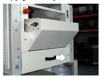
Paper dust and particles accumulate in the paper shredder during operation. To facilitate cleaning, the ground plate of the paper shredder was designed as a tray. This tray must be emptied **every week**.
