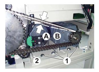
The sagging of the short chain should be 2 to 9 mm in the first month, afterwards 4 to 11 mm, the sagging of the long chain 4 to 11 mm in the first month, afterwards 5 to 15 mm.
