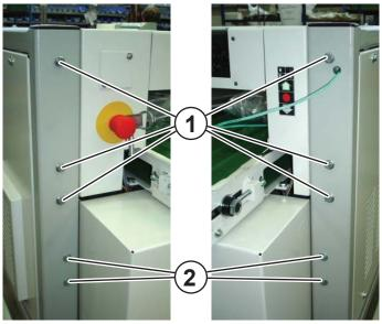
Fasten the supports to the frame with the screws (2).
