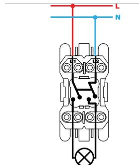
Interruptor bipolar / Double pole switch
