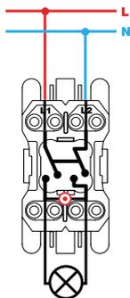
Interruptor bipolar / Double pole switch
