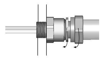
8. Finally, fully tighten the nut (4), into the entry component (1).
