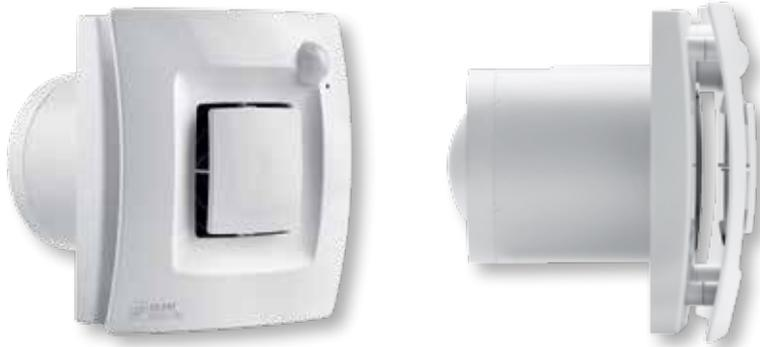
Autonomous and intelligent extractor fan for the bathroom. It automatically adjusts its performance to the ambient conditions and ventilation requirements via a presence detection sensor and a humidity sensor.
