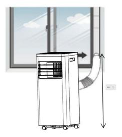
**Step 7:** Adjust the louver at the air outlet, and then switch on the unit.
