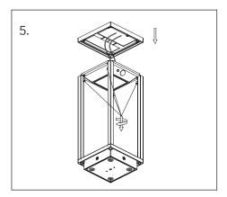
Reconnect the Solar panel lead, then locate the head to the body and refit the 4 screws
