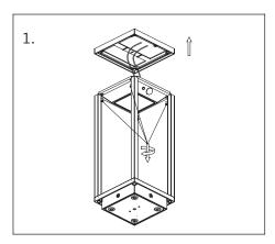
Remove the 4 screws as indicated above to release the top of the body
