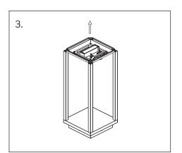
Disconnect and remove the old battery
