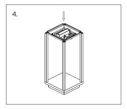
Connect replacement battery and fit into battery holder
