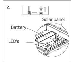
Disconnect the solar panel lead from the top of the body
