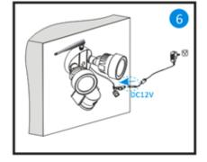
Connect the output of the supplied 12V power adapter into the power socket on the camera.
