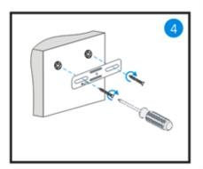
Use a screw driver to screw the crossbar into the chosen surface with the included screws (A).
