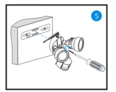
Put the included screw (D) through the center hole of the camera bracket and crossbar. Tighten the screw properly to secure the camera onto the wall.
