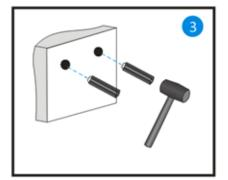
Use a rubber hammer to hit the included plastic plugs into the holes. Ensure the plastic plugs be fixed into the wall without loose.
