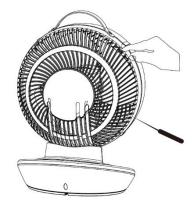
2. Squeeze the two tabs to the left and right of the screws and pull away. At the front of the fan blades there is a locking cap – unscrew the cap in a clockwise motion to remove the fan blades.
