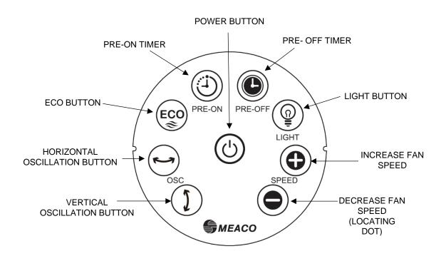
The following functions are only available via the remote control. All other buttons on the remote-control work in the same way as the control panel (see page 5). The remote control has a range of approximately three metres. Before using the remote control, remove the plastic tab.
