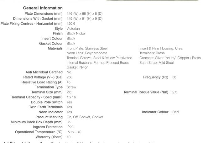
Additional InformationFor cleaning / polishing of products, use only a soft, dry, clean cloth.<br/>Ensure that the mains supply is isolated before commencing installation and refer to the circuit<br/>diagram with the relevant product.<br/>Bare earth cables must always be covered with appropriate sleeving and wired to the earth terminal.
