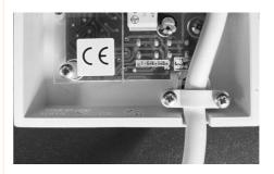
Carefully fit the control plate into the back box ensuring that no wires are trapped during the siting process. Use the two fixing screws to secure to the back box.
