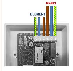
Clamp the element cable to the bottom of the wall controller.
