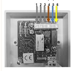
From Left to Right terminals **4-6** correspond to the Mains cable wires.
