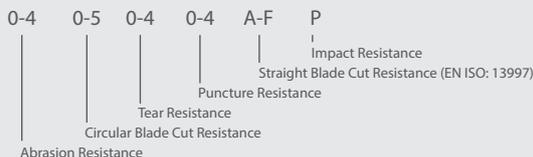
\*If tests are not performed or are not applicable, 'X' will be placed instead of a number/letter
