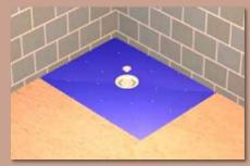
floor drain base component using the  $\frac{3}{4} \times 8$  csk self-tapping crews provided. Then screw in the 1.5" waste fitting using the dust cap. Leave the dust cap in for now. Ensure all the remaining floor drain components are removed
