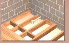
Measure the position of the floor waste trap accordingly, install the waste pipe work in accordance and connect to the trap in an approved manner. Floor Boards removed for illustration purposes.
