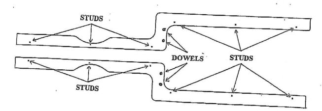
ROUNDED EDGES ON BOTH RAILS MUST BE FACING DOWNWARDS
