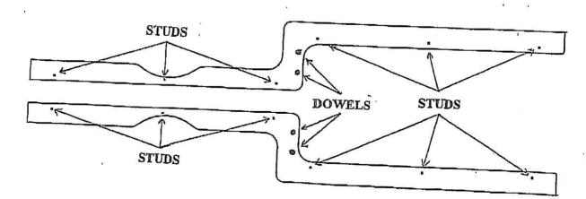
ROUNDED EDGES ON BOTH RAILS MUST BE FACING DOWNWARDS
