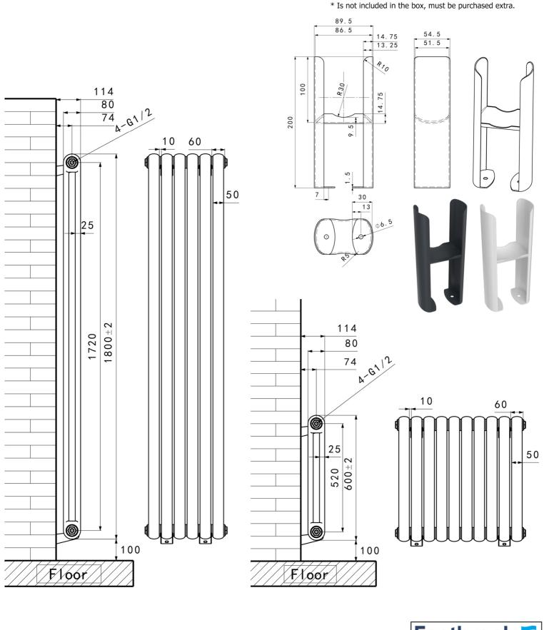
Tappings are the width of the radiator and approx. 74mm off the wall. Distance from wall is 114mm.
