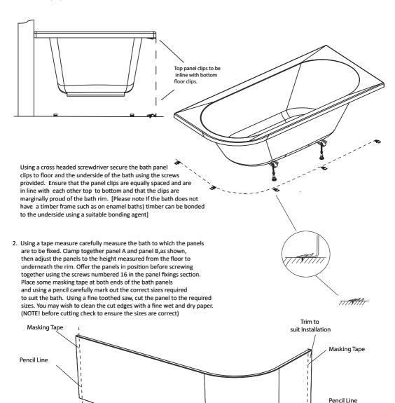
3. Carefully fit the bath panel to the bath by gently pushing the bath panel into place. Ensure that the bath panel is firmly held in place with the bath panel clips.
