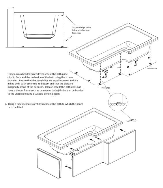
Carefully fit the bath panel to the bath by gently pushing the bath panel into place. Ensure that the bath panel is firmly held in place with the bath panel clips.
