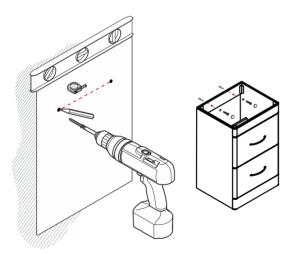
Mark the two holes levelly on the wall.
