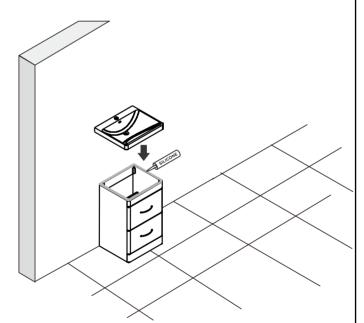
When fitting the basin to the unit, adequate silicone is required between basin and unit to prevent potential water ingress.
