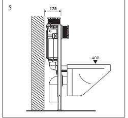
Fix partion wall spacer 4. Fit chosen pan with bolts supplied ensure pan connector, bolts and male flush pipe (B) are left long enough for depth of partion wall and tiles 5. Test flush and check all joints for leaks. Remove pan construct partition wall. It is the responsibility of the installer to ensure an access panel is provided to enable all maintainable parts to be changed without the need for any re-tiling or grouting.
