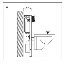
Fit chosen pan with bolts supplied ensure pan connector, bolts and male flush pipe (B) are left long enough for depth of partion wall and tiles ⑤. Test flush and check all joints for leaks. Remove pan construct partition wall. It is the responsibility of the installer to ensure an access panel is provided to enable all maintainable parts to be changed without the need for any re-tiling or grouting
