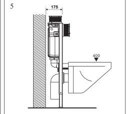
Fix partion wall spacer ④. Fit chosen pan with bolts supplied ensure pan connector, bolts and male flush pipe (B) are left long enough for depth of partion wall and tiles ⑤. Test flush and check all joints for leaks. Remove pan construct partition wall.
