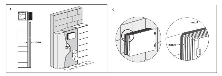
Tile partion wall 6 ensuring tiles are within 5mm of partion wall spacer.
