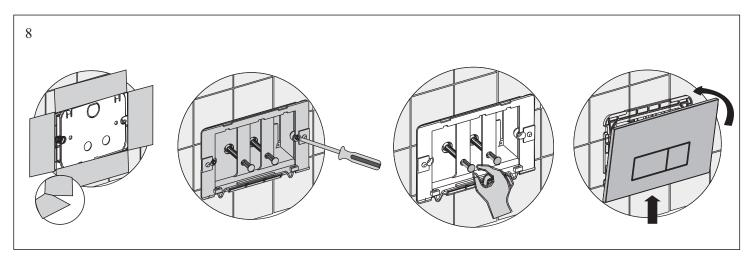
$Fit flush \ plate \ bracket. \ Push \ rods \ should \ screw \ up \ to \ smooth \ shoulder, \ trim \ accordingly \ and \ install. \\ Fit flush \ plate \ (supplied \ separately) \ .$
