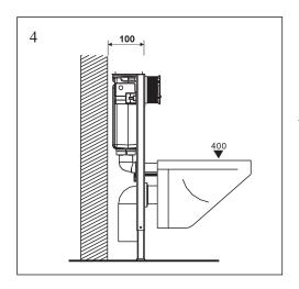
Fit chosen pan with bolts supplied ensure pan connector, bolts and male flush pipe (B) are left long enough for depth of partion wall and tiles ⑤. Test flush and check all joints for leaks. Remove pan construct partition wall.
