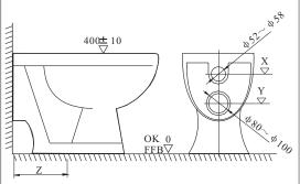
Measure the height from the centre of fill pipe to the floor X, the height from the centre of flush pipe to the floor Y before install.
