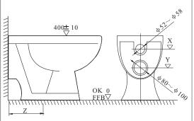
Measure the height from the centre of fill pipe to the floor X, the height from the centre of flush pipe to the floor Y before install.
