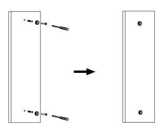
Drill 2 holes (Distance is 650mm) in desired position.
