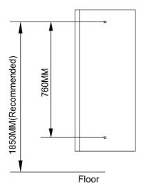
Drill a hole (size as above) in the wall. The distance is based on the products.
