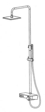
Remove the protective cap from the showerhead ball joint and screw the unit onto the overhead arm ensuring the filter washer is in place. This arm is not adjustable.
