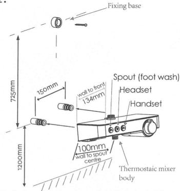
Push the S connector into the two holes in the back of the Thermostaic mixer body to make it close to the wall, and then tighten the screw on the bottom of the main body by allen key. The wall bracket recommended height of 725mm, fixing it with screws.
