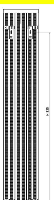
Rear wall brackets positioning for 4, 5 and 6 panel vertical sizes (410mm, 510mm and 610mm width)
