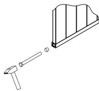
\* Diverter should be installed into the flow side of the radiator
