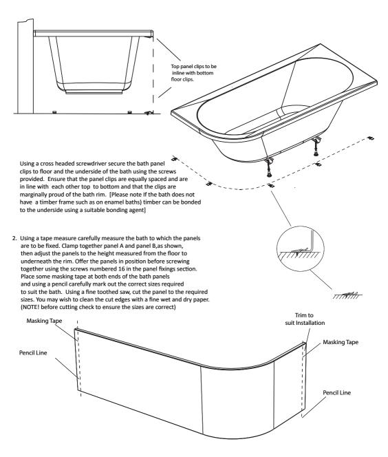
3. Carefully fit the bath panel to the bath by gently pushing the bath panel into place. Ensure that the bath panel is firmly held in place with the bath panel clips.
