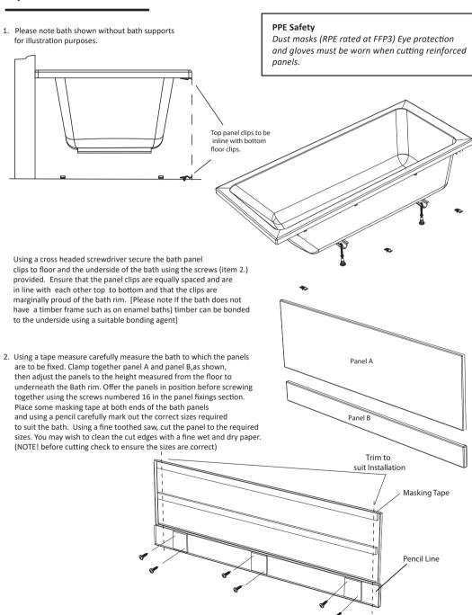
3. Carefully fit the bath panel to the bath by gently pushing the bath panel into place. Ensure that the bath panel is firmly held in place with the bath panel clips.
