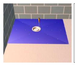
Drill and screw the floor drain base component into place using the ¾ x 8 csk self tapping screws provided. Then screw in the 1.5" waste fitting using the dust cap. Leave dust cap in place for now. Ensure all the remaining floor drain components are removed.
