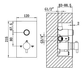
Step 1: recommended installation depth for the concealed valve body.
