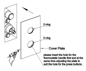
Step 2: Before installing the cover plate to the wall please lubricate the Orings with silicone grease (or similar) to prevent scratching during fitting. Then apply clear silicone sealant around the back edge of the cover plate and carefully press into the position (please insert the hole for the thermostatic handle first and at the same time adjusting the plate to suit the hole for the press buttons).
