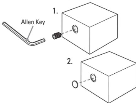
Attach the grub screw to the spindle and secure in position. Place the cover cap on the handles to cover the holes.
