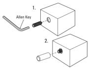
Attach the handle to the temperature spindle and secure in position so that when the valve is at its hottest, the handle arm is pointing towards the 'HOT' marking on the cover plate.
