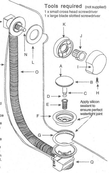
Knob to check that the plug 'pops up' sufficiently to allow the water to be drained from the bath. Tighten the nut (item C).
