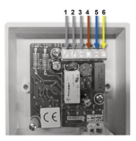
From Left to Right terminals 4-6 correspond to the Mains cable wires.
