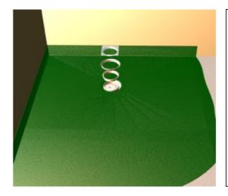
Insert the membrane clamp, height adjustment ring, height extension ring (where necessary) and stainless steel frame.
