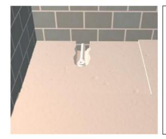
Fit the waste pipe and shower trap as required. The waste pipe should be solvent welded to the shower trap outlet.
