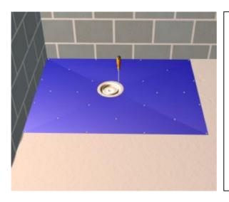
Drill and screw the floor drain base component into place using the  $\frac{3}{4}$  x 8 csk self tapping screws provided. Then screw in the 1.5" waste fitting using the dust cap. Leave dust cap in place for now. Ensure all the remaining floor drain components are removed.
