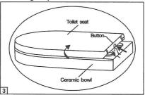
Press the button to release toilet seat from ceramic bowl and open toilet seat to make it in vertical position.
