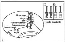
Install expansion nut,rubber washer, hinge and bolt into hole of ceramic bowl, tighten them by screwdriver, then cover the hinge cap at last.
