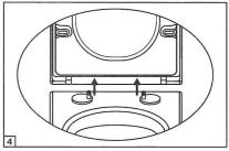
4. Lift up toilet seat to disassemble it.
