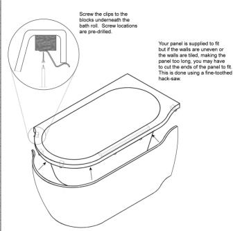
Insert the panel into the clip starting at one end of the bath and continue all the way round to the other end.
