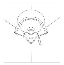
4) Put the expanding plastic into the hole, then fix the bolt with 60mm out of the hole.
