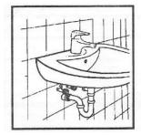
2. Temporarily place the half-pedestal against the basin and mark the mounting positions on the wall.
