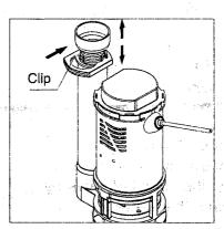
2. Slid the clip as per the picture, adjust the height of overflow pipe as you need. Put the clip back.
