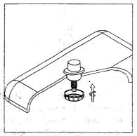
2.Insert the button into the oval hole of tank and then screw up the flanged nut.
