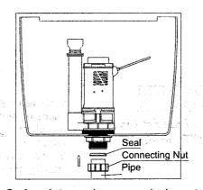
2. As picture shown, orderly put the connecting nut and seal on the pipe, then insert the pipe into the flush valve hole.
