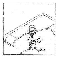
3. Push in switch box's green clip (1) to connect with the button body.
