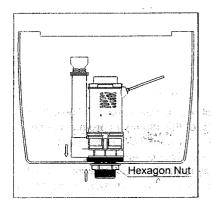
1. Insert the flush valve in the tank hole from inside. Adjust it to the proper place and tighten the hexagon nut from outside.
