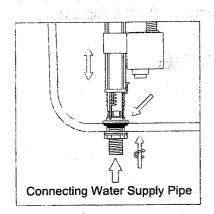
4. Position the fill valve in the water tank, screw the washer and nut. Please take a note that the valve should not touch with anything.
