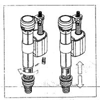
1. Uninstall the plug, turning the valve in anticlockwise. Adjust the height of valve by pushing the valve up and down.
