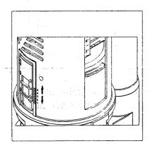
1. Adjust the full flush volume by sliding the full flush adjuster up and down.
