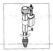
2. Turn the valve in clockwise and install the plug.
