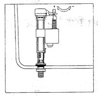
5. Adjust the water level by screwing the adjustment bolt, the water level should be under the overflow level not less than 2cm.
