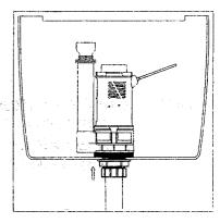
3. Screw the connecting nut to make sure the pipe is attached tightly to the flush valve.
