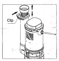
2. Slid the clip as per the picture, adjust the height of overflow pipe as you need. Put the clip back.
