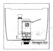
1. Insert the flush valve in the tank hole from inside. Adjust it to the proper place and tighten the hexagon nut from outside.
