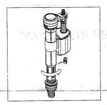
2. Turn the valve in clockwise and install the plug.
