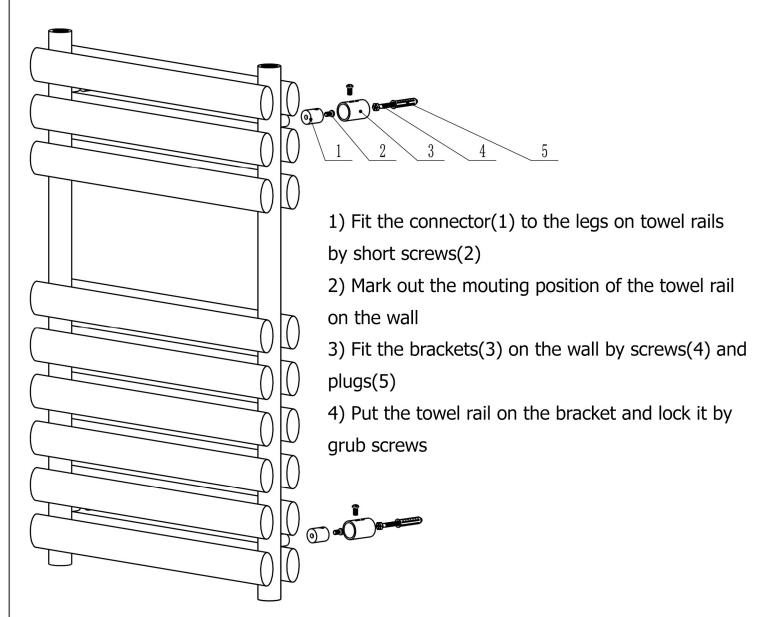
Maximum working pressure of this radiator is 4 bar. This radiator is to be used on Domestic Central Heating systems only. (Not suitable for use on direct hot water systems)
