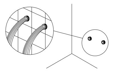
Before assembly, flush the water supply pipes thoroughly to remove debris (allow the water to run with the main stopcock open for about 3 mins), otherwise dirt particles might affect the function of the shower panel!
