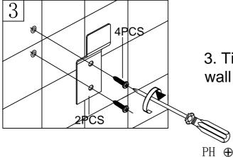
3. Tighten the screws to the wall with wall mounting brackets.
