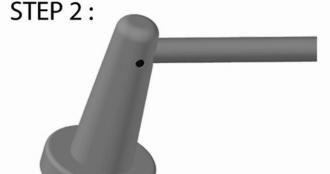
To shorten the hanging bar, please remove both brackets by loosening the grub screws with the allen key provided. If the bar does not need to be shortened, please tighten grub screws before installing as they are not fully secured during assembly in case of adjustment.
