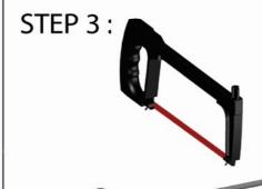
Cut bar to required length using a good quality metal saw. When cutting to length, please check bar is length required with the brackets attached.
