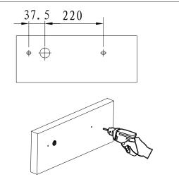
1, Drill two holes in  $\phi$  5mm according to the image shown.
