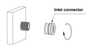
2. Screw the inlet connector like image shown.
