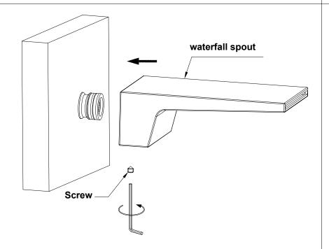
3. Install the waterfall spout and then tighten it by screw.
