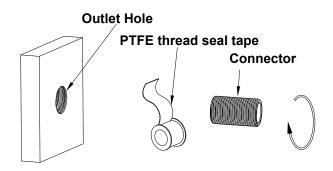
1. Wrap PTFE thread seal around the connector, and then screw it to the outlet hole.
