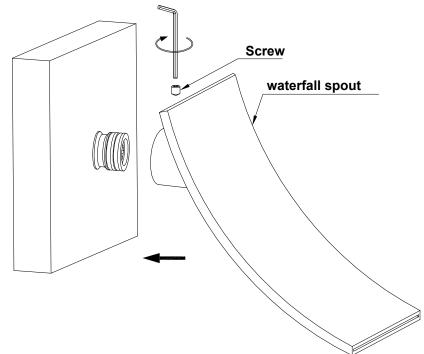
3. Install the waterfall spout and then tighten it by screw.
