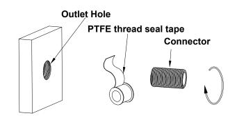
1. Wrap PTFE thread seal around the connector, and then screw it to the outlet hole.
